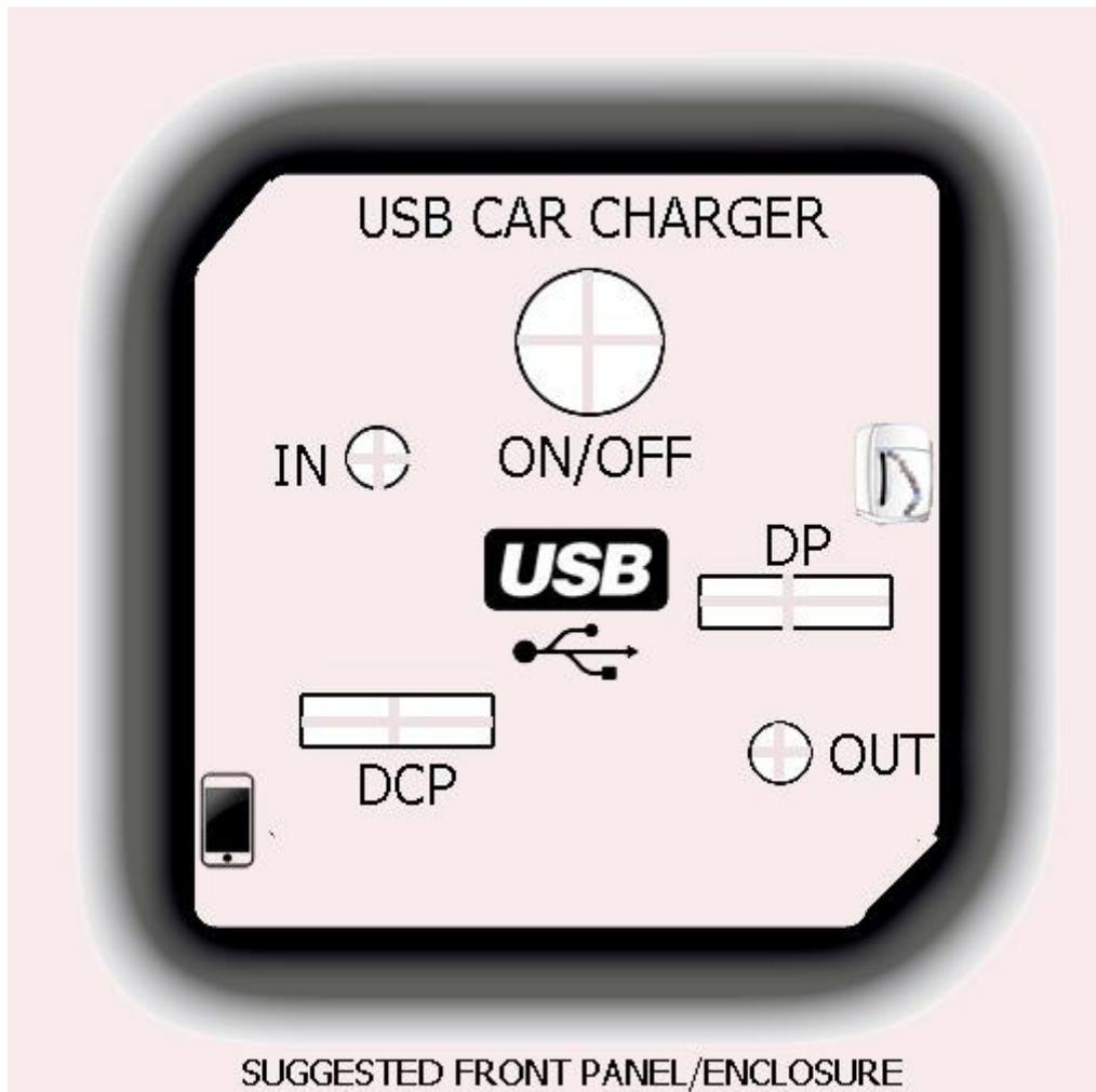
Building up the usb car charger should not present undue difficulties if you follow the components list and (ofcourse) the datasheets of crucial components used. It is recommended to build the system on a small circuit board. Having verified the circuit works properly, you are ready to fit the wired circuit board in a suitable enclosure with the suggested front panel. The enclosure may be finished to individual taste.
